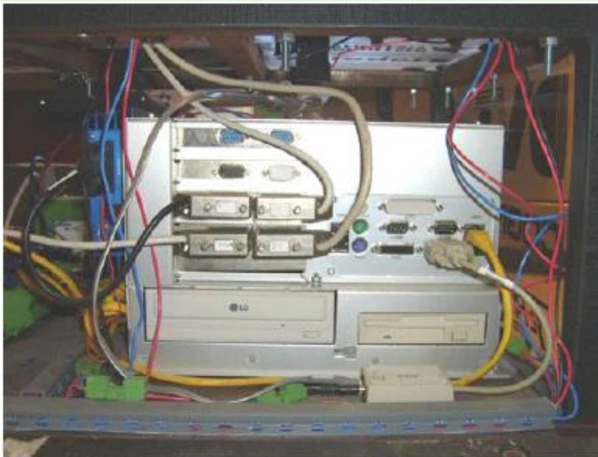
Fig. 2. Phoenix Contact IPC5500 Industrial PC, fully connected.
