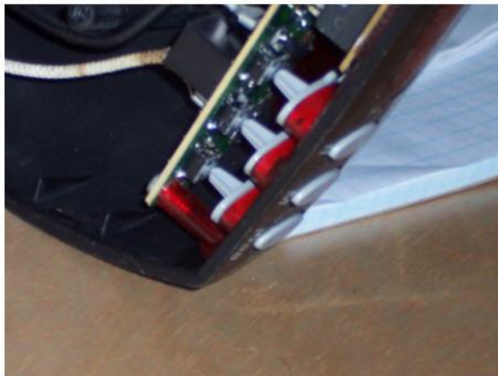
PCB switches in a cheap coffee maker.
