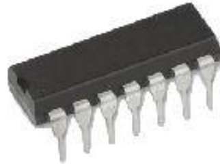
Digital Logic Gate (Chip Package)
