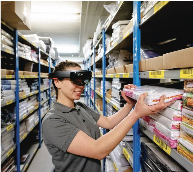
Figure 2: Microsoft HoloLens in use in a warehouse facility in The Netherlands [3]
