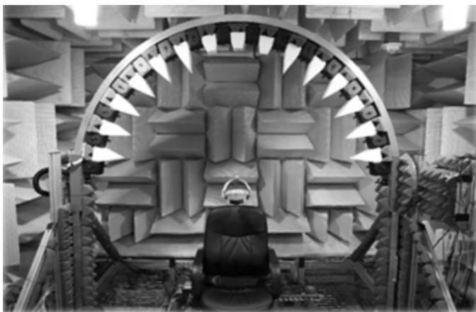
Figure 6: Head-related transfer function measurement setup in Microsoft Research [10]
