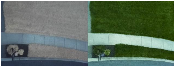
Left: Raw image from NoIR camera module with blue filter. Right: Raw image from normal camera module.
