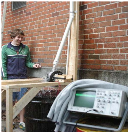
Ryan Cohick demonstrates his team's pumped hydroelectric energy storage system that pumped water to the roof of Esbenshade and recovered electrical energy through a custom turbine and alternator.
