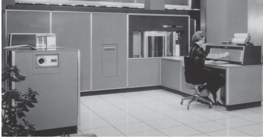
FIGURE 6.14.2 The RAMAC disk drive from IBM, made in 1956, was the first disk drive with a moving head and the first with multiple platters. The IBM storage technology Web site has a discussion of IBM's major contributions to storage technology.
