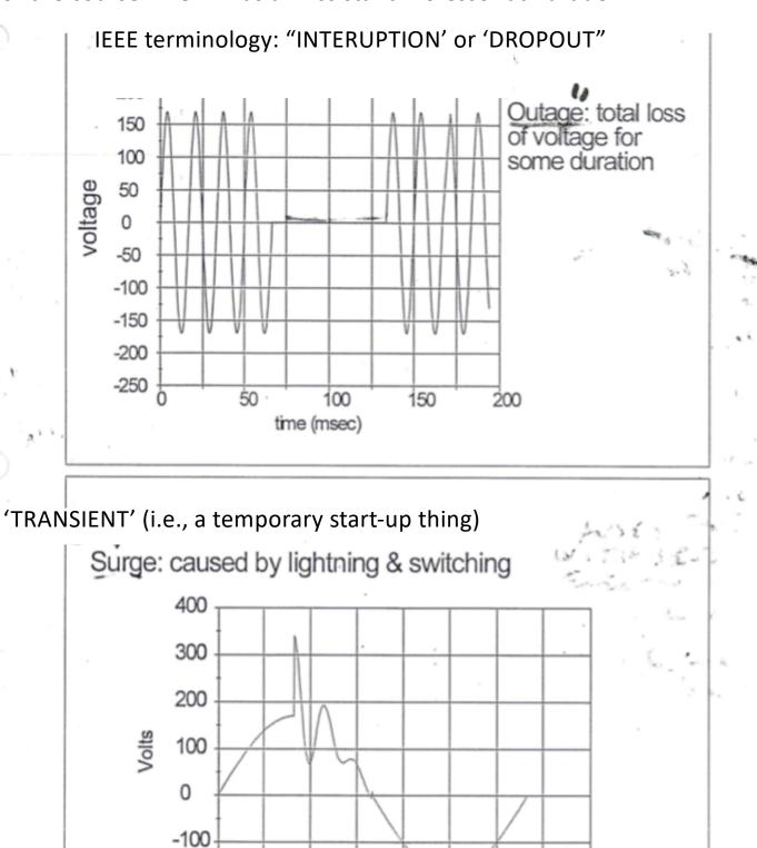
EXAMPLE CAUSES: 1) initial energizing of power factor correction capacitors 2) switching on transmission lines
