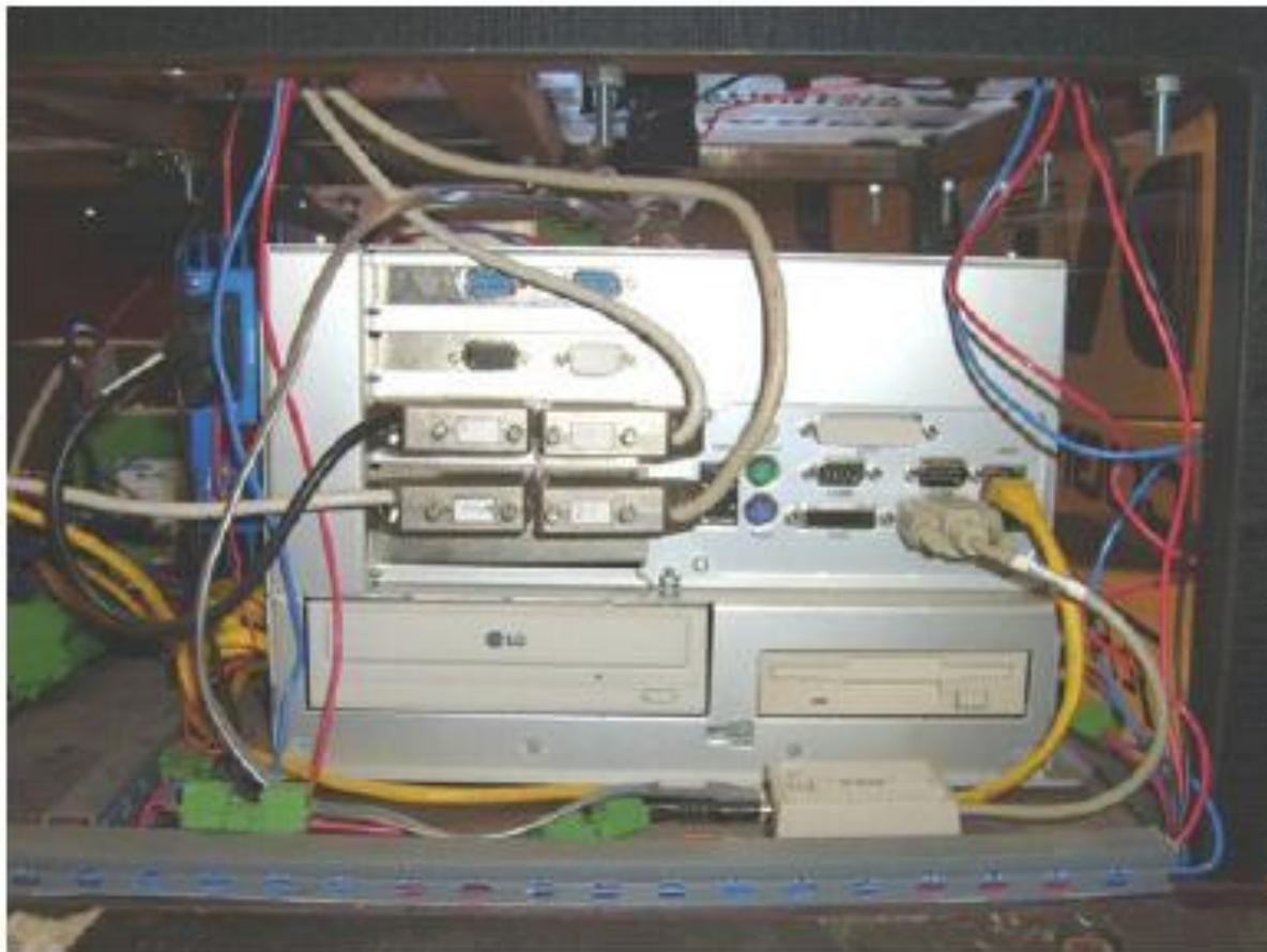
Fig. 2. Phoenix Contact IPC5500 Industrial PC, fully connected.
