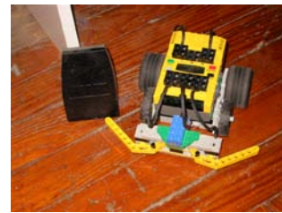
Figure 4: IR Tower and Scout Robot. The robot must face the tower in order to communicate with the Simulation.
