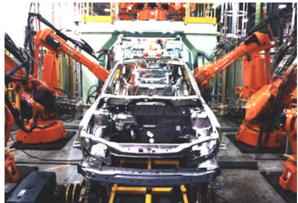
Figure 2. Robots assembling unibody [1].
