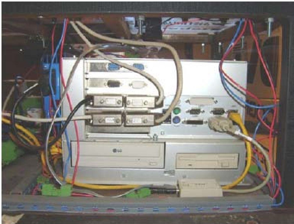
Fig. 2. Phoenix Contact IPC5500 Industrial PC, fully connected.
