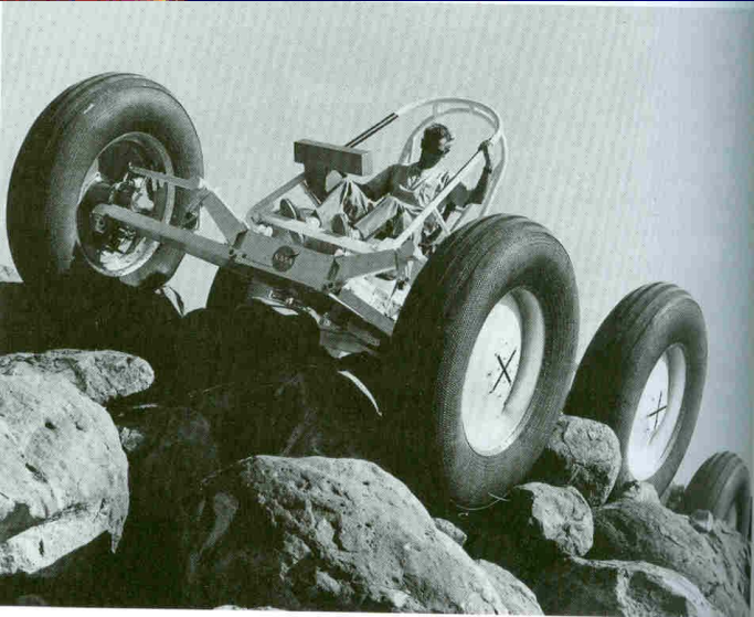
General Motors' Defense Research Laboratories (GM-DRL) division performed extensive vehicle mobility studies for NASA during the 1960s as well. This MTA built by DRL is shown traversing a boulder obstacle field. (NASA/MSFC)
