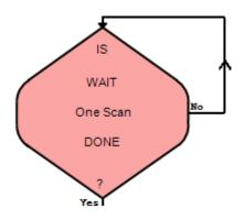
Lastly, the wait block is used for pauses in the flowchart. An example would be for turning on a light bulb for 5 seconds before shutting off. It defaults to one scan wait, but a scan is something less than a second long, so it is often necessary to change it to seconds.
