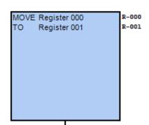
This is a simple example moving the data from register 000 to register 001.
