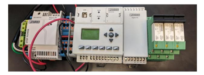
The NanoLC has 4 main modules that are used the in early labs. They are the **Power Unit**, **Main Unit**, **Digital IO Unit**, and **Relays**
