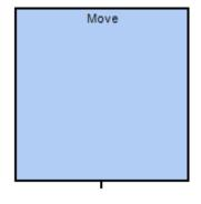
The move block is used for moving the location of data. This is helpful for moving data into registers for storage.
