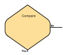
Going through the list of available function blocks, the first one is the compare block. Obviously, it compares two items and outputs a signal to either yes or no depending on what the answer is. Place a block and double click on it to edit it's settings.
