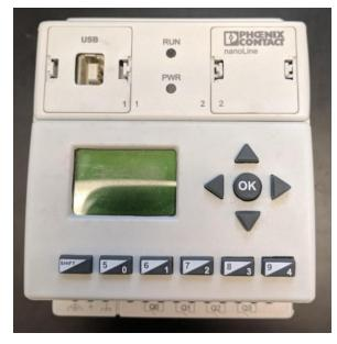
The Main Unit houses the computational components of the NanoLC. This is where you can control the rest of the modules, and will upload your programs. The unit itself houses a control panel, inputs, and outputs. For some projects this and the power unit will be all that is necessary. Located on the top of the unit is the inputs, and a common ground. On the bottom of the unit is the power connectors, and the outputs.
