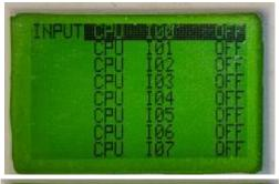
By pressing 0, we enter a menu that shows the status of all of the inputs. In this picture, all of the inputs are currently OFF.
