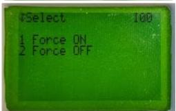
By pressing OK on one of the inputs, another menu shows the options to manually force them ON/OFF, which can be very useful for debugging and testing.
