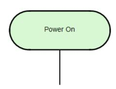
The first function block shown at the top left of your flowchart will always be the power on block. This block is a simple if-statement for if the power is on, then run the program.
