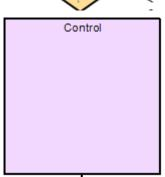
Next, we have the control function block. This block is used for changing binary data items or controlling clocks/counters. This block is often used for turning on/off outputs. Double click on the block to edit it's settings.
