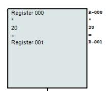
Here is an example of multiplying register 000 by 20 and storing it in register 001.
