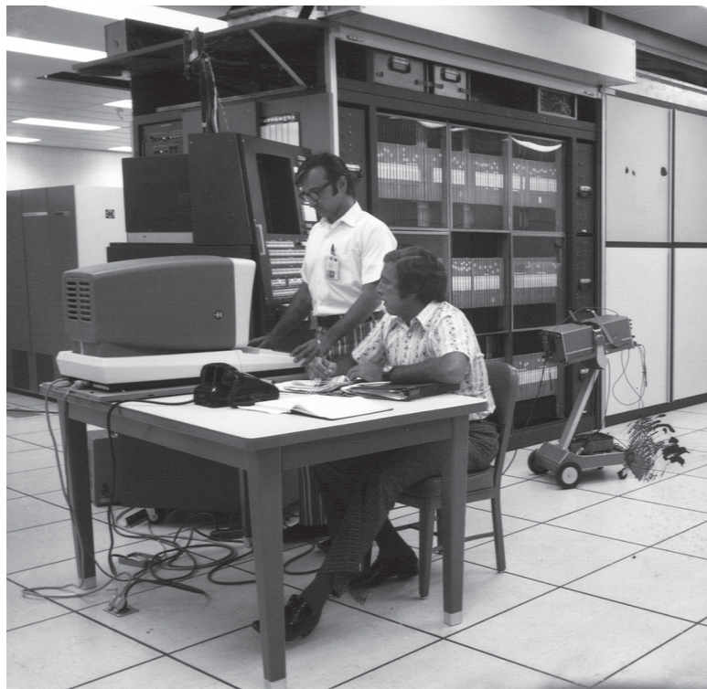
FIGURE 7.14.1 The ILLIAC IV control unit followed by its 64 processing elements. It was perhaps the most infamous of supercomputers. The project started in 1965 and ran its first real application in 1976. The 64 processors used a 13-MHz clock, and their combined main memory size was 1 MB: 64 \times 16 KB. The ILLIAC IV was the first machine to teach us that software for parallel machines dominates hardware issues. Photo courtesy of NASA Ames Research Center.
